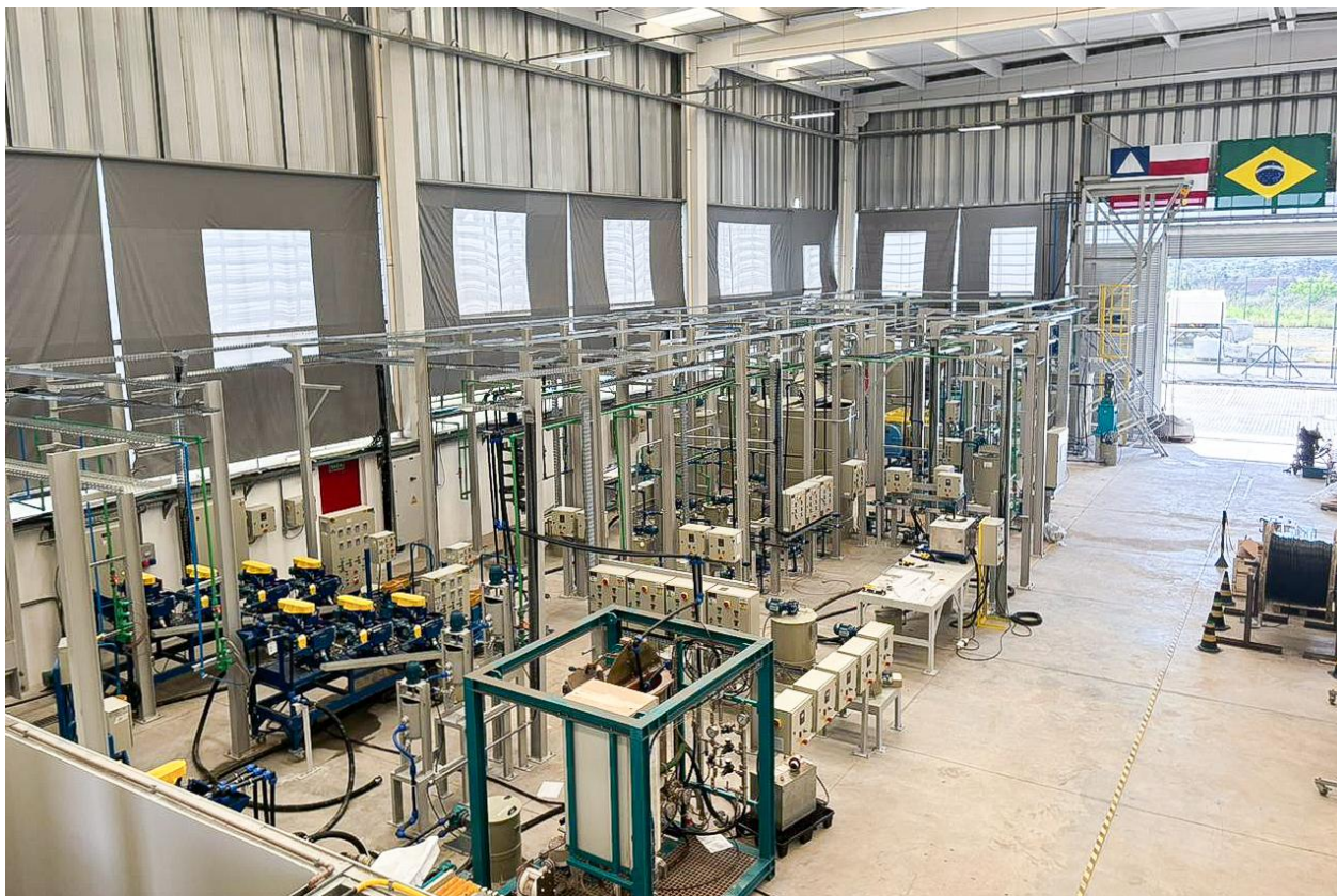
Figure 4: Stage 1 Beneficiation Facility Overview - 100 kg/h Capacity.
