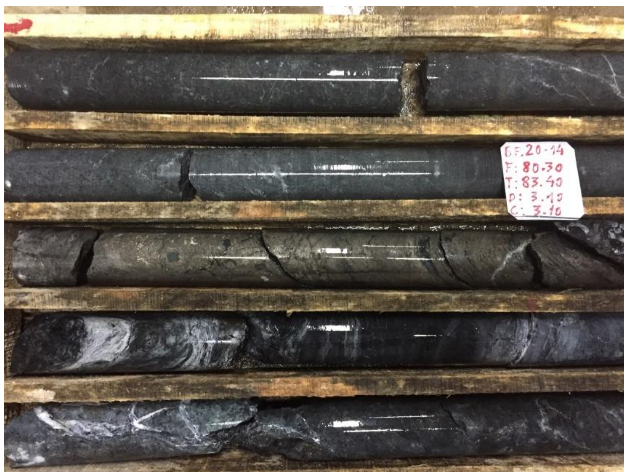
Figure 1: Blackstone drillhole BP20-14 intersects 0.55m of Massive Sulfide Vein (MSV) mineralisation from 83.0m within a 2.5m zone of tremolite-rich dyke within the broader 58m down hole intersection of disseminated sulfide (DSS) at the King Cobra Zone (KCZ)
