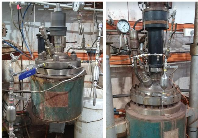
Figure 1.6, Batch POX autoclaves (2 L - left, 15 L - right)
