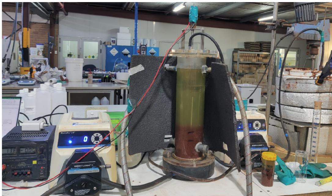
Figure 1.7, Dynamic thickening setup
