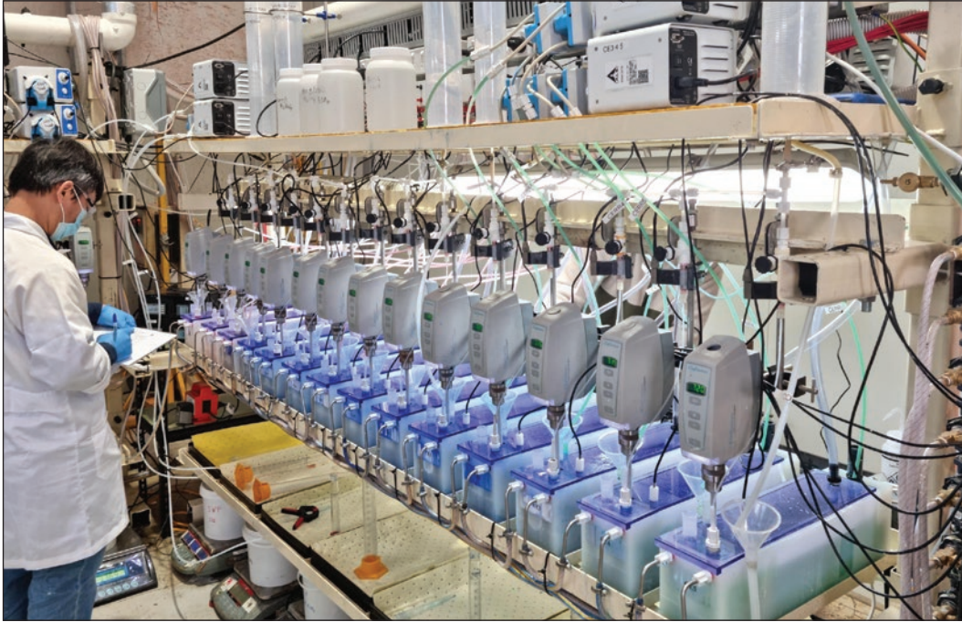
Figure 11 - Pilot Scale Cobalt solvent extraction
