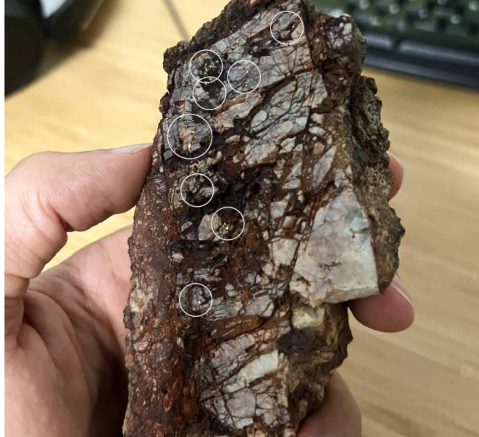
Rock chip sample assaying 66.9 g/t Au (visible gold circled), sample number HG48. Refer to ASX release of 3 December 2024 for full details on these results
