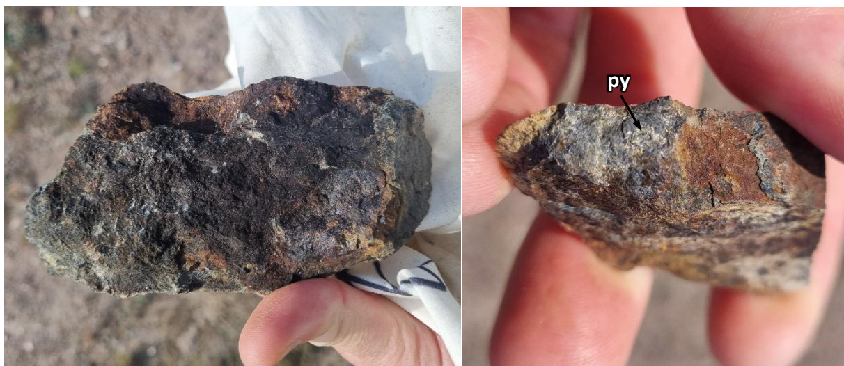
Figure 3: (Top Left) Field photograph LHNS05, chlorite-altered mafic rock with suspected fine disseminated black pitchblende that assayed 1.2% ( U_3O_8 ) from Gyrfalcon; (Top Right) Field photograph LHNS04, mafic rocks with visible pyrite sulphide (py) from Gyrfalcon that assayed 0.57% ( U_3O_8 ) and 1.0% Mo;
