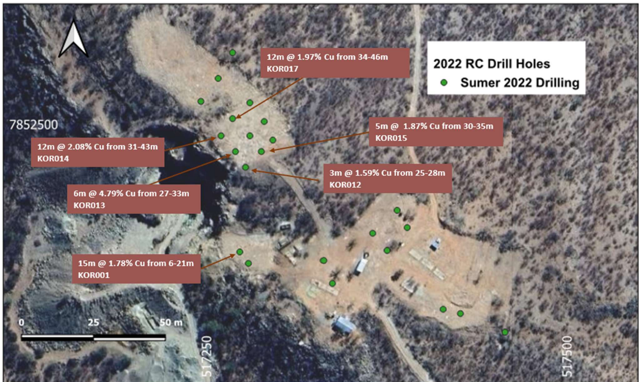
Figure 4: Drill Hole Plan with significant intersections highlighted from drilling in 2022 (see Appendix 2. Refer to Appendix 1 for full details of the intersections).
