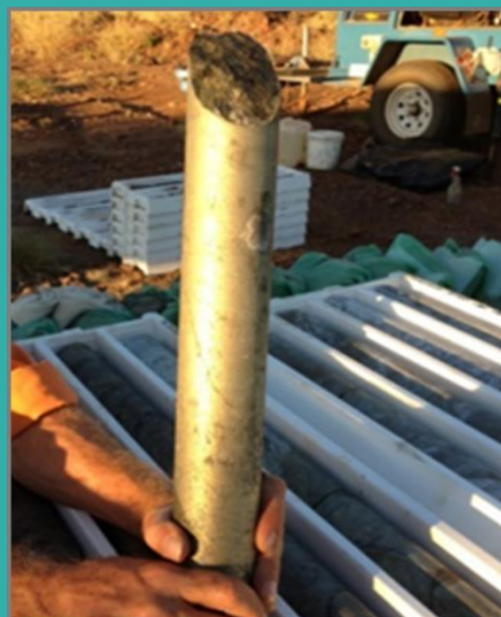
Massive chalcopyrite from main orebody, Drillhole: HCDD0001
