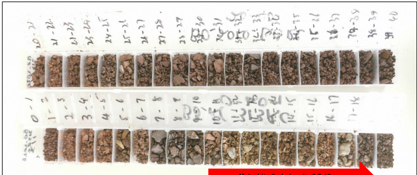
FIGURE B2: HIGH GRADE VISIBLE COPPER MINERALISATION – 313RC FROM 9.5-18m
