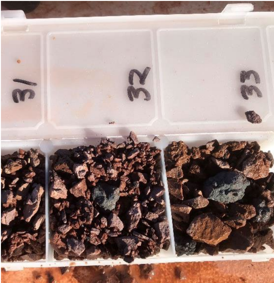
FIGURE C-5: SULPHIDE MINERALISATION IN BO_333RC CHIPS
