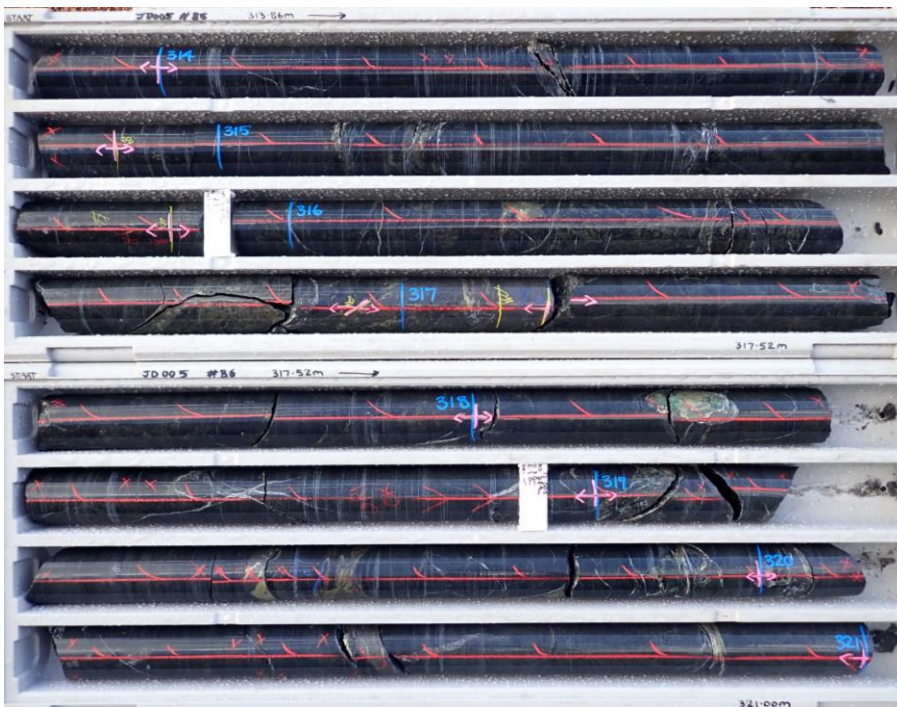
G4 Zone core photos from JD005 (314-321m), ~80m south of JD006 – 10.1m @ 2.9g/t Pd, 0.6g/t Pt, 1.2g/t Au, 0.1% Ni, 1.3% Cu, 0.01% Co
