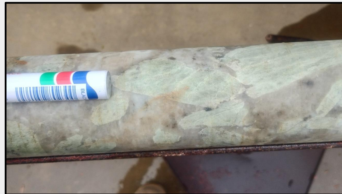
Coarse-grained spodumene in drill core from CLMDD001
