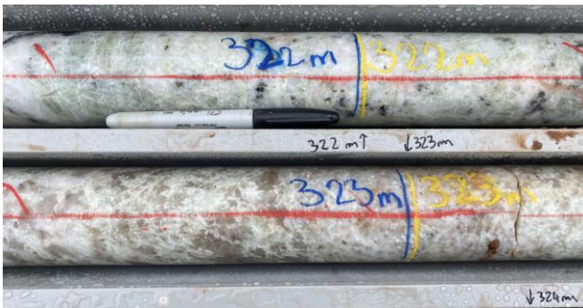
Photograph 3. Zoomed in photo of coarse-grained spodumene in drill core from CLMRC064DT from 322m (with visual estimate of 10 to 25% spodumene mineralisation).
