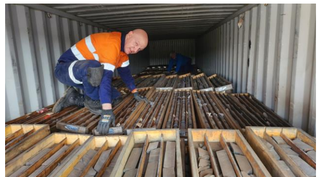
Image 2 - View of inside of sea container – with the drill core stored in trays.
