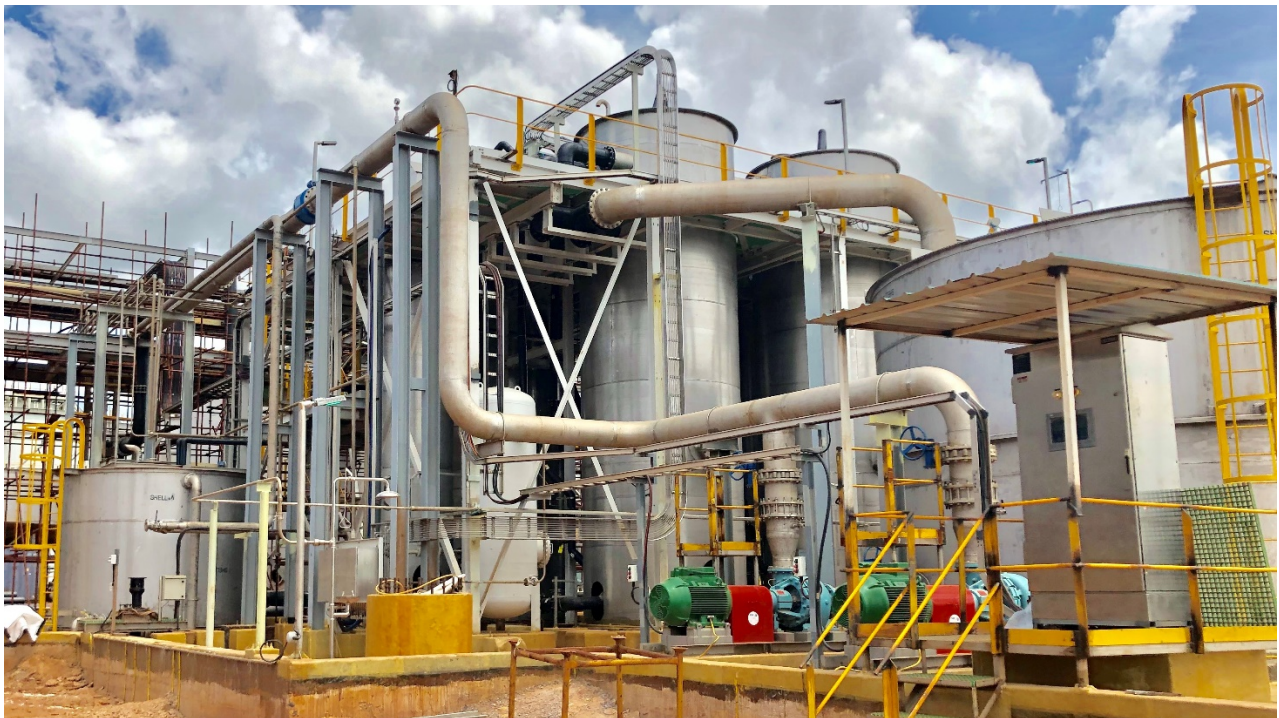
Photo of the CLX Plant in DRC for removal of impurities from a 20,000 tons/day cobalt liquor
