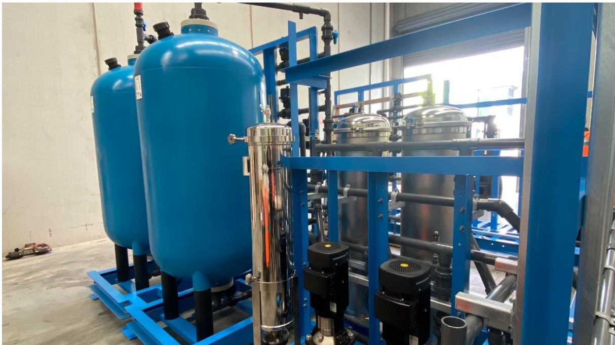
One of the two batch ion exchange skids ready for shipping to site
