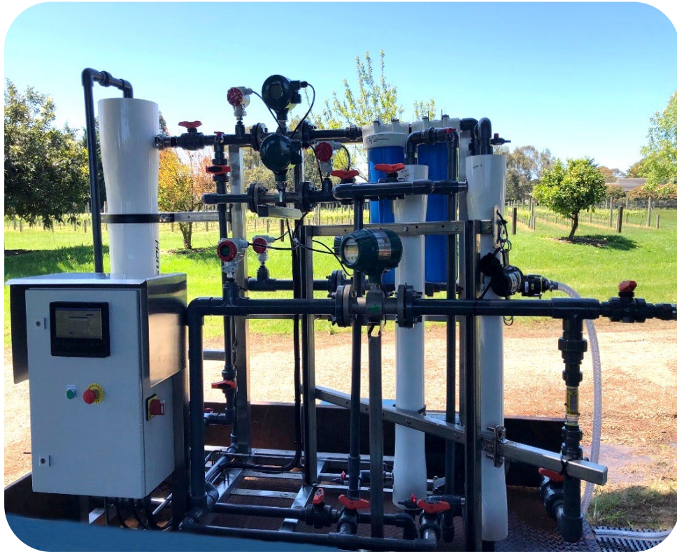
Portable pilot plant for initial field trials of industrial sized 4040 and 8040 NematiQ graphene membranes
