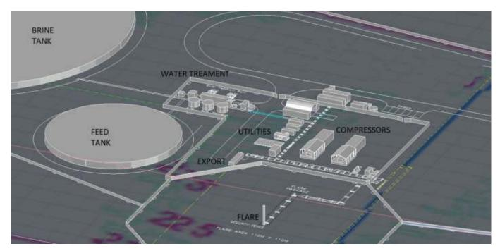
Figure 5 – Conceptual layout of facilities planned for Mahalo North
