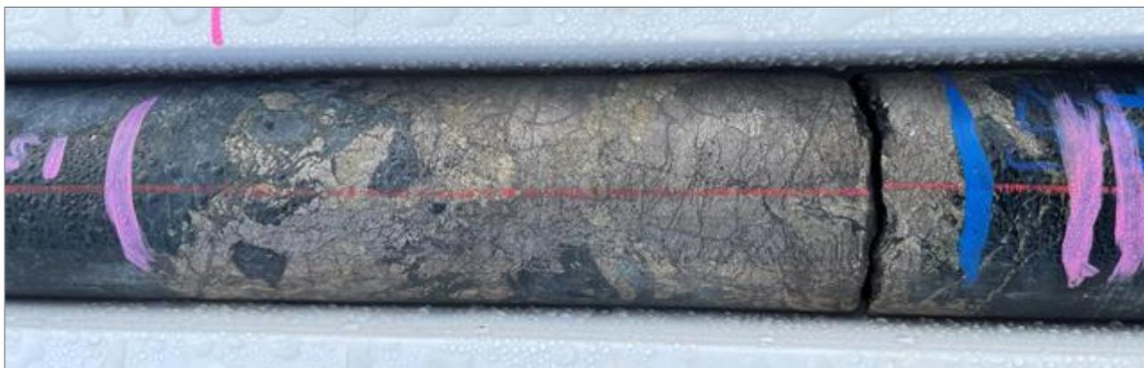
Figure 2. Mineralisation at 156.1m in YAD0017, assaying 4.17g/t PGE (0.95g/t Pd, 3.22g/t Pt), 3.49%Ni & 1.43% Cu.
