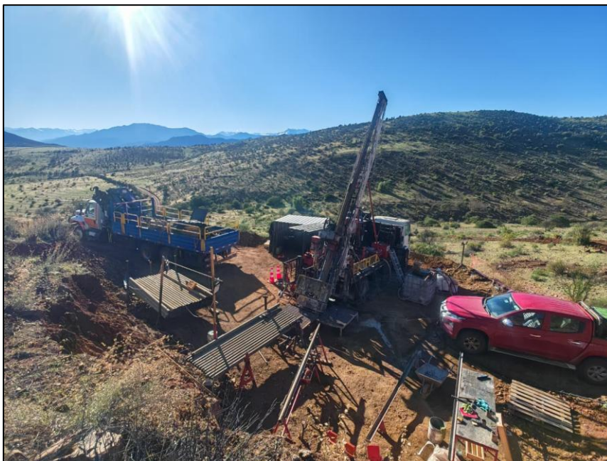
Figure 6: Drill rig drilling maiden diamond hole CMQD001 at El Quillay West.
