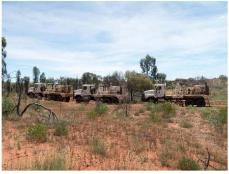
Figure: Seismic vibrator array in Southern Amadeus Basin providing energy to image sub-surface horizons
