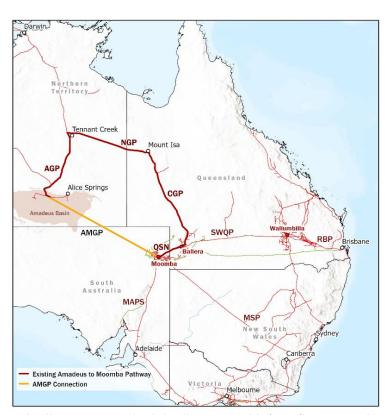
The AMGP is planned to be a 950km pipeline, up to 16-inch in diameter with free-flow capacity of 124TJ per day (45PJ per year), and would be expandable with compression.
