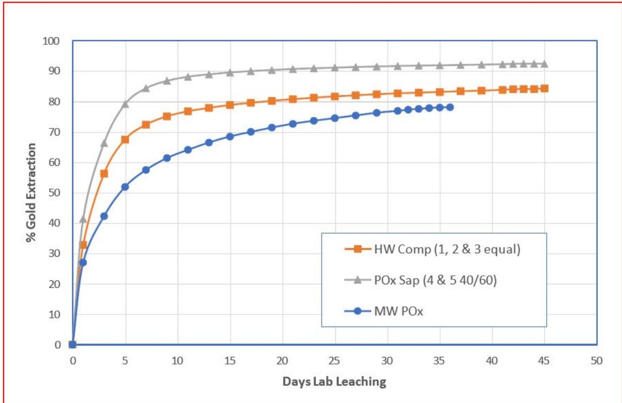
**Figure 1: Column Test Recovery Curves – Gold**
