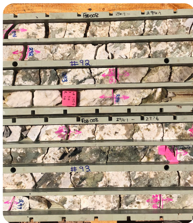
Spodumene pegmatite drill core from Finniss Lithium Project.
