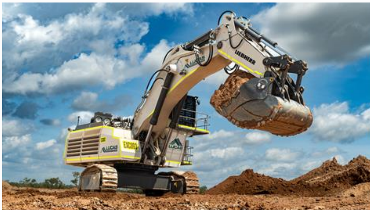
Figure 3. 210 tonne Liebherr R9200 excavator at Core's Finnis Lithium Project, NT
