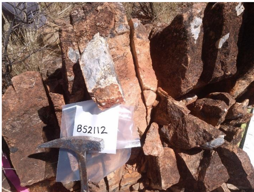
Figure 3: Spodumene bearing pegmatite assaying 4.78% \text{Li}_2\text{O} at Bismark
