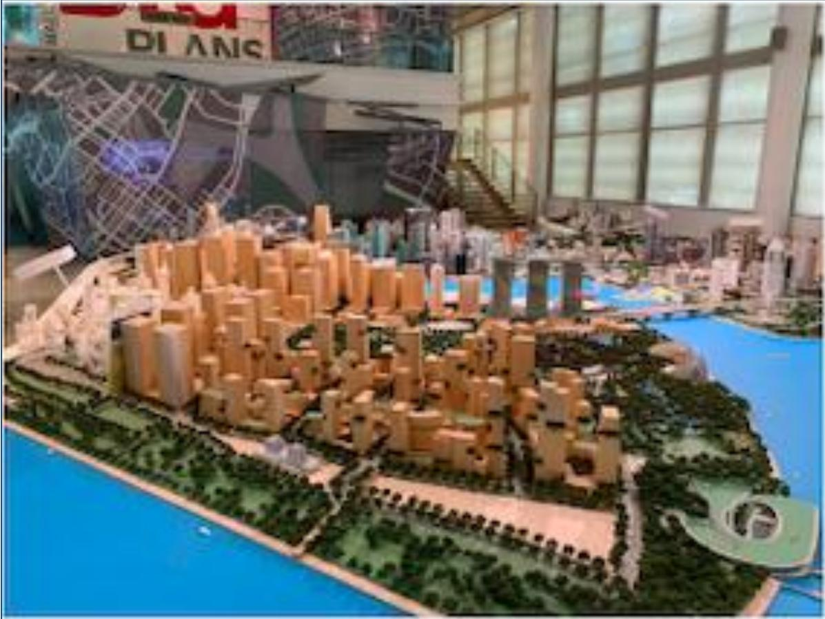
**Figure 4:** Plan model showing the planned construction on the reclaimed Jurong island in Singapore's harbour depicted in Figure 3. Not only is the land being built on reclamation sand, the concrete used in the building construction planned comprises ~30%-40% construction sand, illustrating the sand requirement for this form of development found in the high growth regions of the world.
