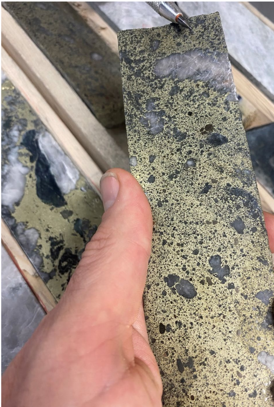
Image 1: High grade drill core from CB-24-100 intersecting 7.3m @ @ 4.2% Cu, 0.3g/t Au & 16.6g/t Ag. Image showing core between 321.9m and 322.6m.
