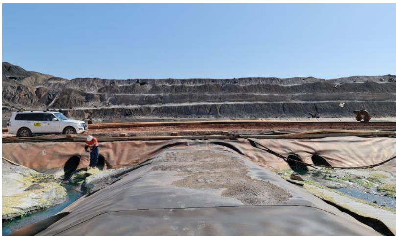
Image 2 / Leach Solution from Heap Drains – twin drains of copper sulphate solution
