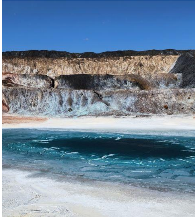
Image 1 / Copper Leaching from Heaps – blue is copper sulphate
