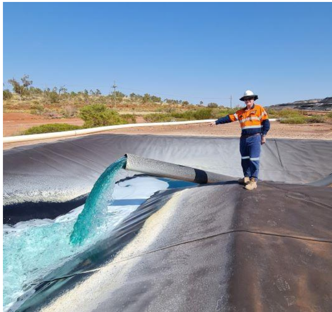
Image 3 / Leach Solution pumped from collection ponds to PLS pond – blue copper sulphate solution
