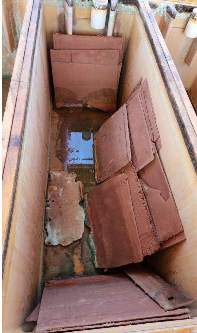
Image 4 / Copper cathode to be recovered from the bottom of an EW cell after removing cathodes and anodes – red metal plates
