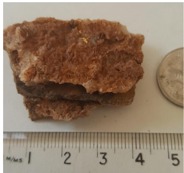
Fig 2 Photographs of the gold nuggets being recovered from the core of the Top Camp area (216 nuggets for 36 grams) and an example of a gold particle intergrown with laminated vein consisting of a core of iron-oxide and a margin of lighter coloured quartz and carbonate (photos are provided by P Gower and the gold is not the property of Coziron Resources Ltd).
