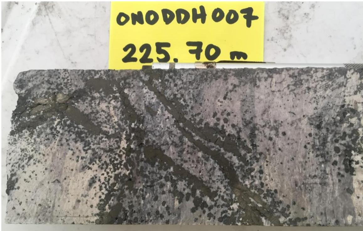
**Figure 6 -** Altered and mineralized volcanic host rock with up to 7% metallic sulphide in drill hole ONODDH007, HQ core from 355.5 m depth - Ono Island Project, Fiji.
