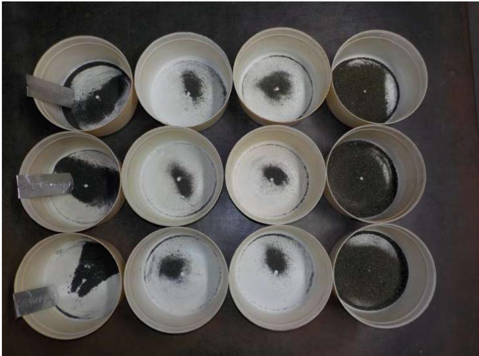
**Plate 3** – Magnetic to non-magnetic (left to right) heavy minerals from WHIMS processing
