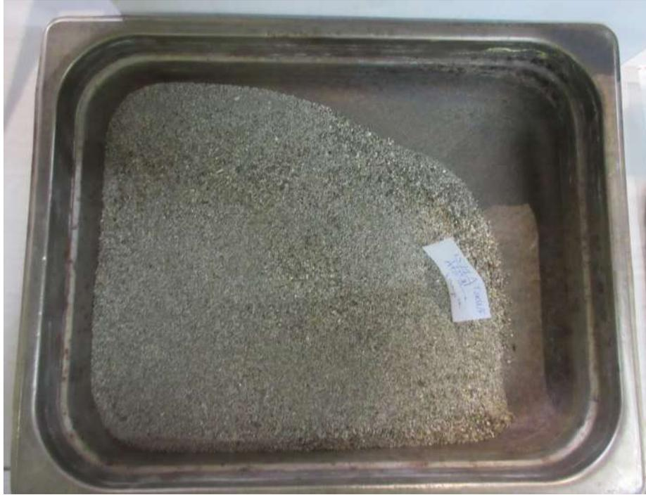
**Plate 4** – Washed coarse and finer industrial sand after removal of the magnetite and heavy minerals
