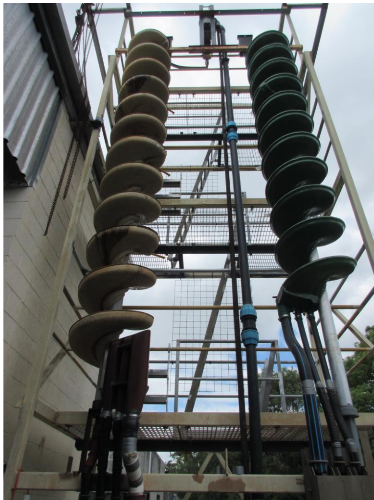
Plate 1 – Spirals used to separate heavy minerals from bulk sand samples, during metallurgical testing at IHC Robbins metallurgical facility in Brisbane.
