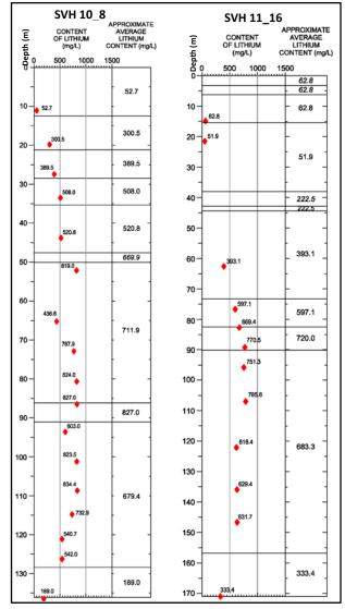
Figure 3: Lithium One (Galaxy) drillholes SVH10\_8 & SVH11\_16 noting near surface Li versus underlying economic Li grades (ref: Lithium One NI43-101, March 2012)
