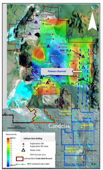
Figure 2: Base gravity/aerial foto image showing eastern palaeochannel, location of Lithium One (Galaxy) drilling & DMI Samples – Candelas area (ref: Lithium One NI43-101, March 2012)
