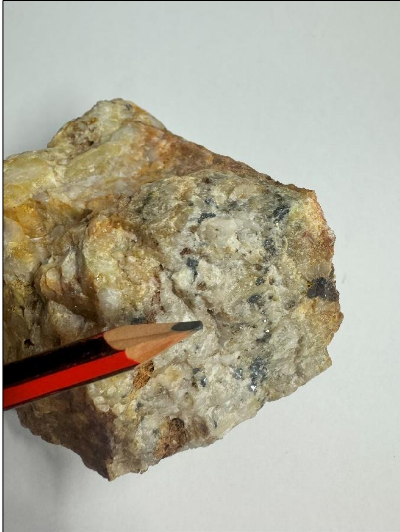
Figure 4: Grab sample (Sample ID: 217558) from the Antimony Mine showing veinlet of Antimony within quartz veining.
