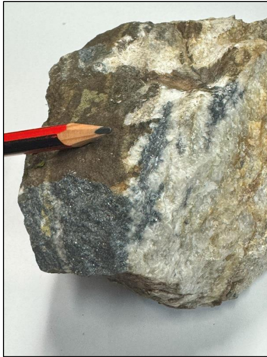
Figure 1: Grab sample (Sample ID: 217566) from the Carry On mine waste dump showing massive sulphide antimony mineralisation (grey mass on left of image) within quartz veining.
