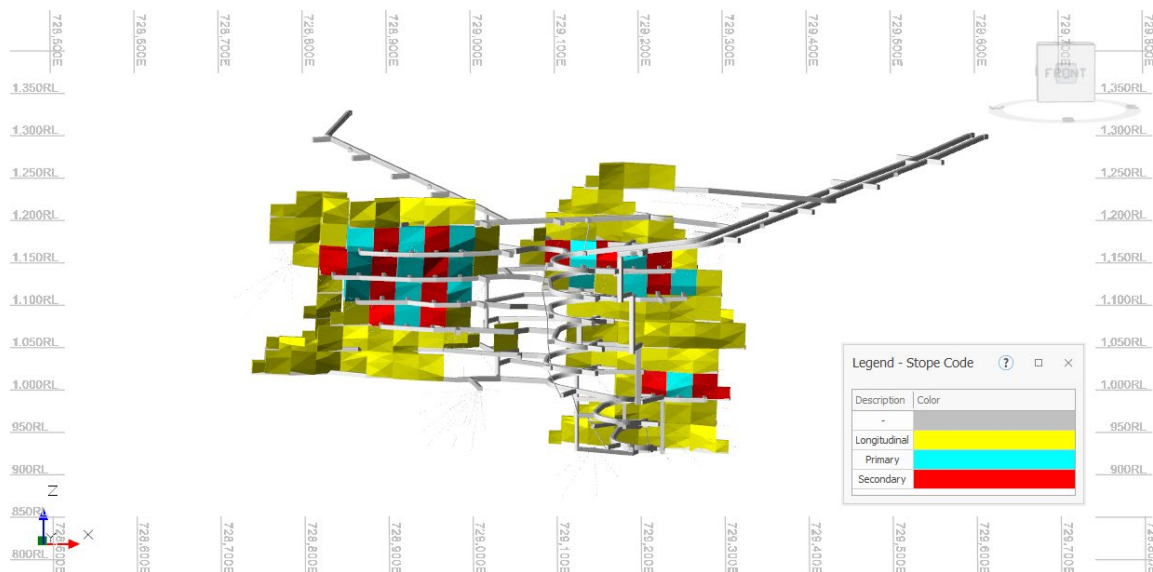
Figure 8 Sulphur Springs's stope mining methods
