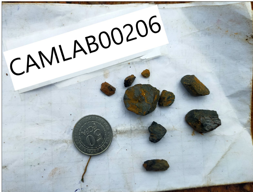
Figure 2: The rutilite nuggets display a massive texture, with some grains exhibiting elongation. The rutilite displays a sub-metallic lustre with dark grey to black colour with minor secondary Fe-oxide coating and sub-rounded crystal suggesting limited lateral transport. XRF results in Table 2 and Appendix II.
