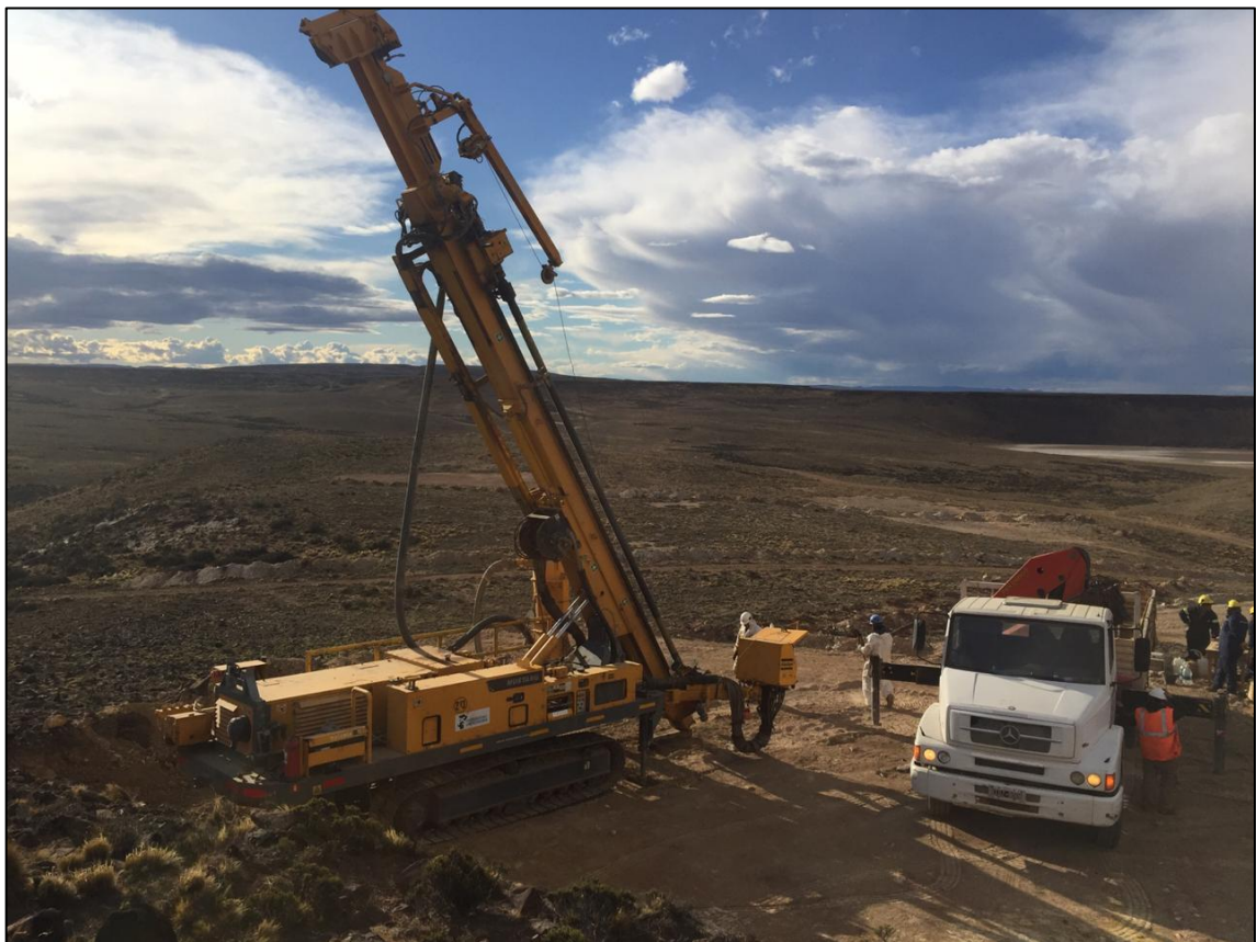
Figure 2: RC drill rig on site at Veta Blanca
