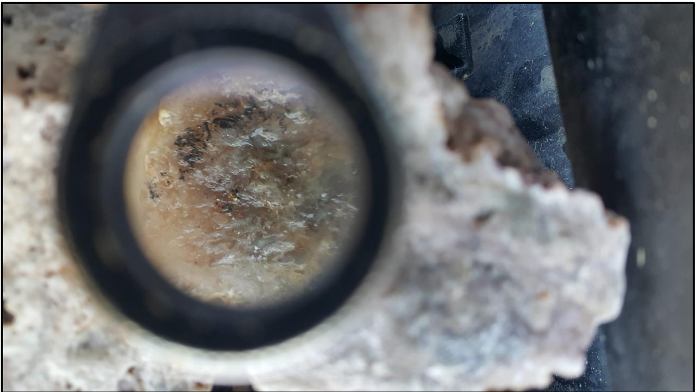
Figure 3: Magnified view of visible gold (electrum?) in sample 11951 returning 40.4gpt Au
