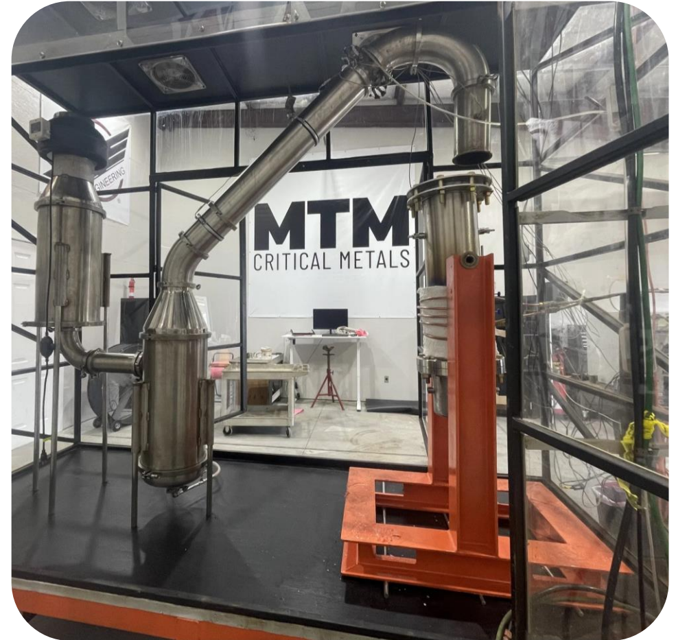
Metallium Ltd — Flash Joule Heating reactor (test unit).
