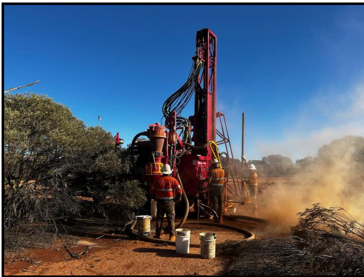
Figure 5: Fenceline aircore drilling in progress at Revere
