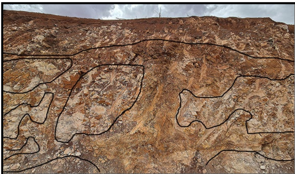
Figure 12: Alteration arsenic rich mineralised halo in bulk sampling trench grading 0.4g/t, looking northeast
