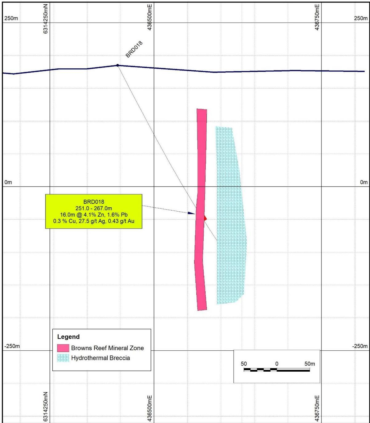
**Figure 7** Interpreted cross section 6314 200N through the Browns Reef deposit showing the drill hole trace for hole BRD018.
