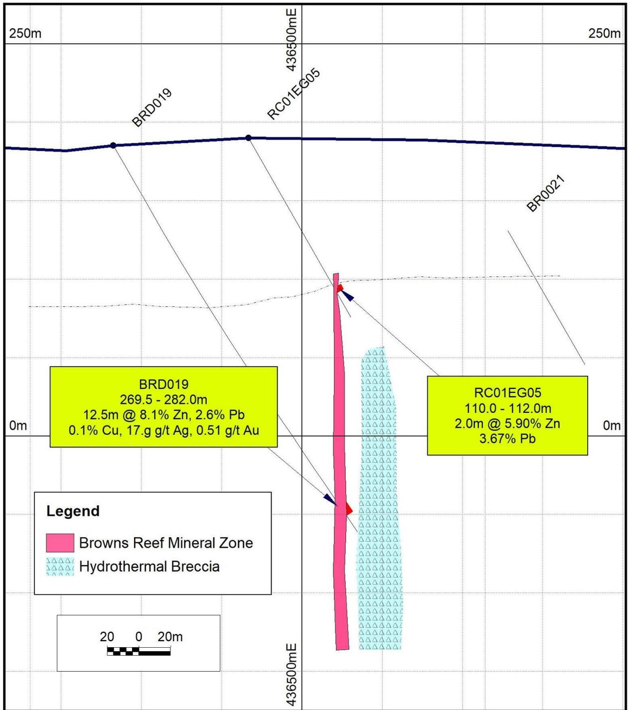
**Figure 8** Interpreted cross section 6314 300N through the Browns Reef deposit showing the drill hole traces for previous hole RC01EG05 and hole BRD019.
