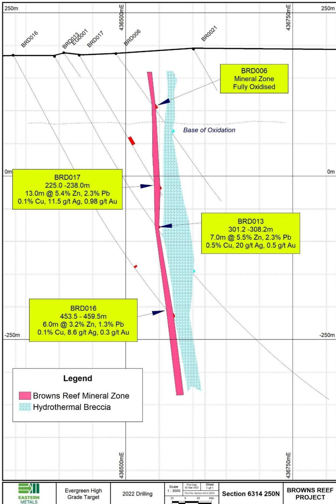
**Figure 6** Interpreted cross section through the Browns Reef deposit showing previous drill hole traces and holes BRD016 and BRD017.
