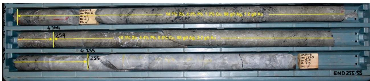
**Figure 4** Massive sulphide mineralisation in drill core from hole BRD018 253.0m-255.5m.
