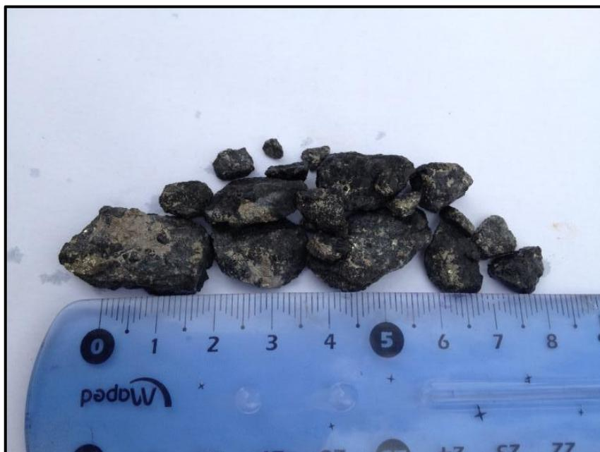
**Plate 1. Selected drill chips, PLRC002, Interval 225-226m**
