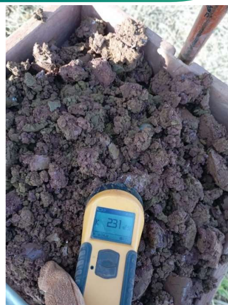
Figure 6: Magnetic susceptibility of drill cuttings at CDE-AD-0006 hole in CODA East
