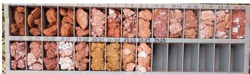
Figure 5: Auger drill cutting chip library of CDE-AD-007 auger hole
