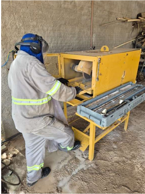
Figure 4: Splitting of core received from EAS-DD-0001
