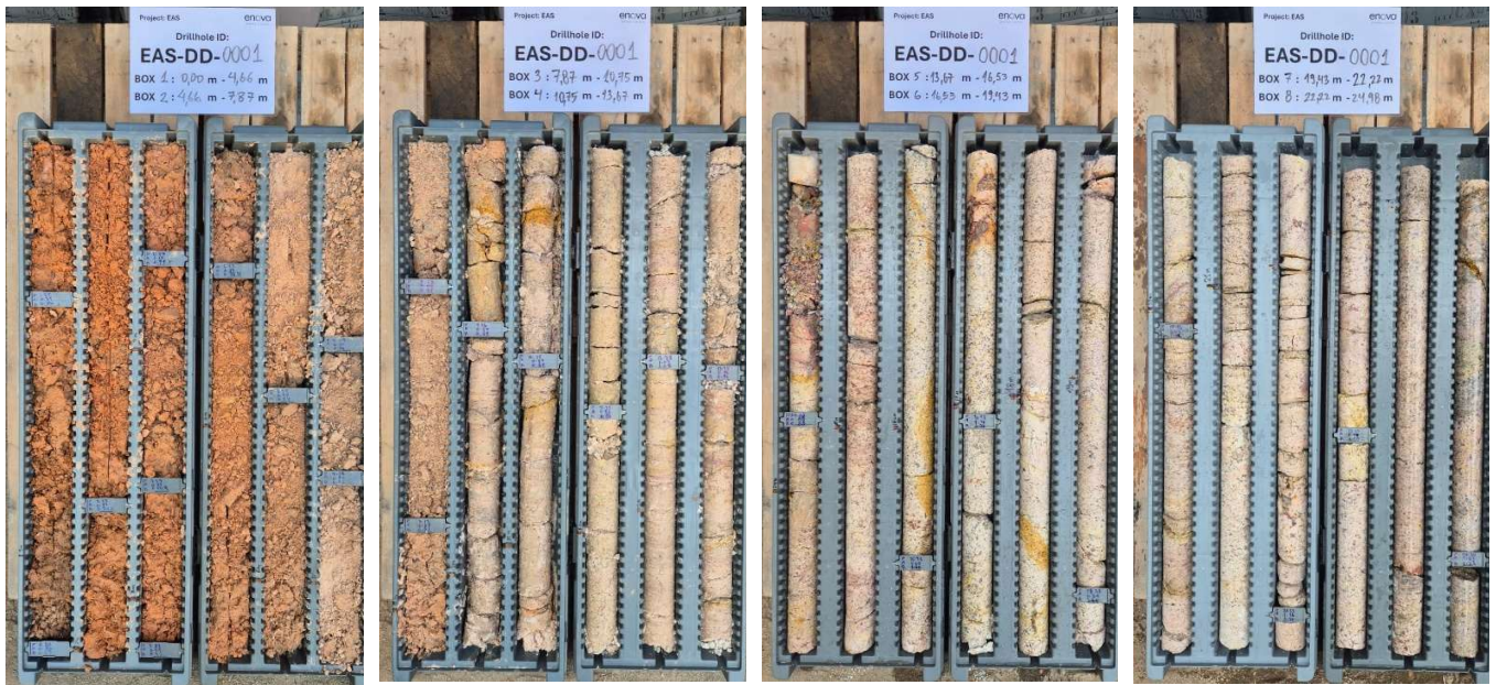
Figure 6: Saprolite clay in EAS-DD-0001 diamond hole
