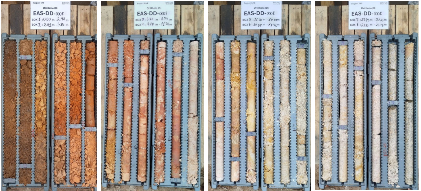
Figure 6: Saprolite clay in EAS-DD-0008 diamond hole
