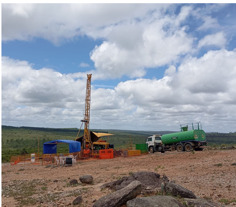
Figure 3A and 3B: Diamond drill rig at hole EAS-DD-0007.
