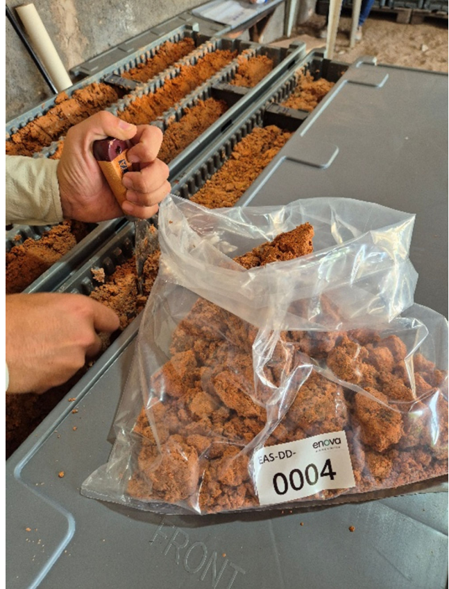
Figure 5: samples are packed and tagged prior to dispatch to laboratory
