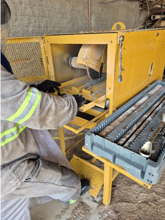
Figure 4: Splitting core with diamond saw
