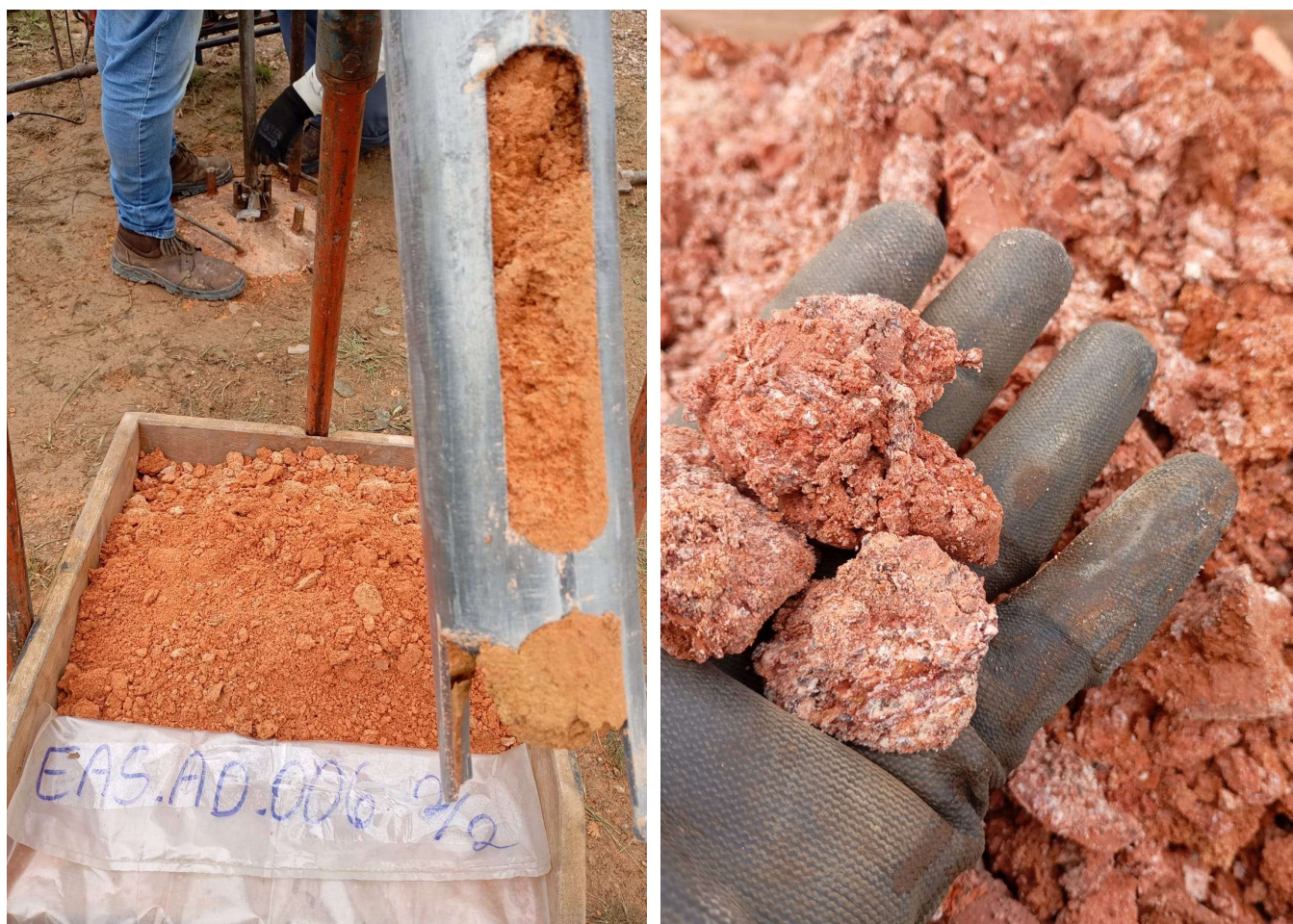
Figure 3 and 4: Auger Saprolite Sample EAS.AD.006 at hole EAS-AD-0001
