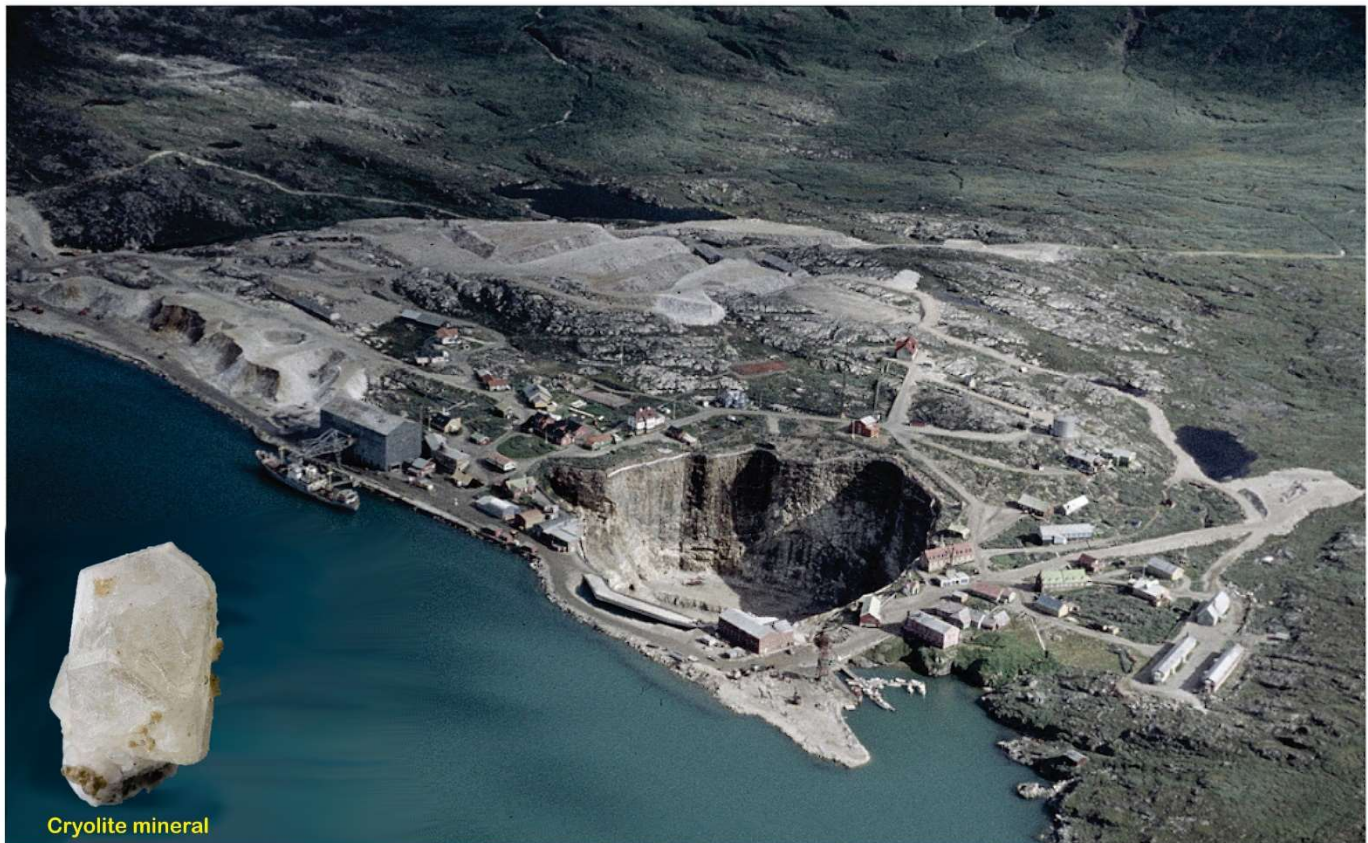
Figure 1: Aerial image of Ivittuut and the cryolite mine in 1960, showing the working open-pit, mine infrastructure, ore and waste dumps and ship loading facilities.
