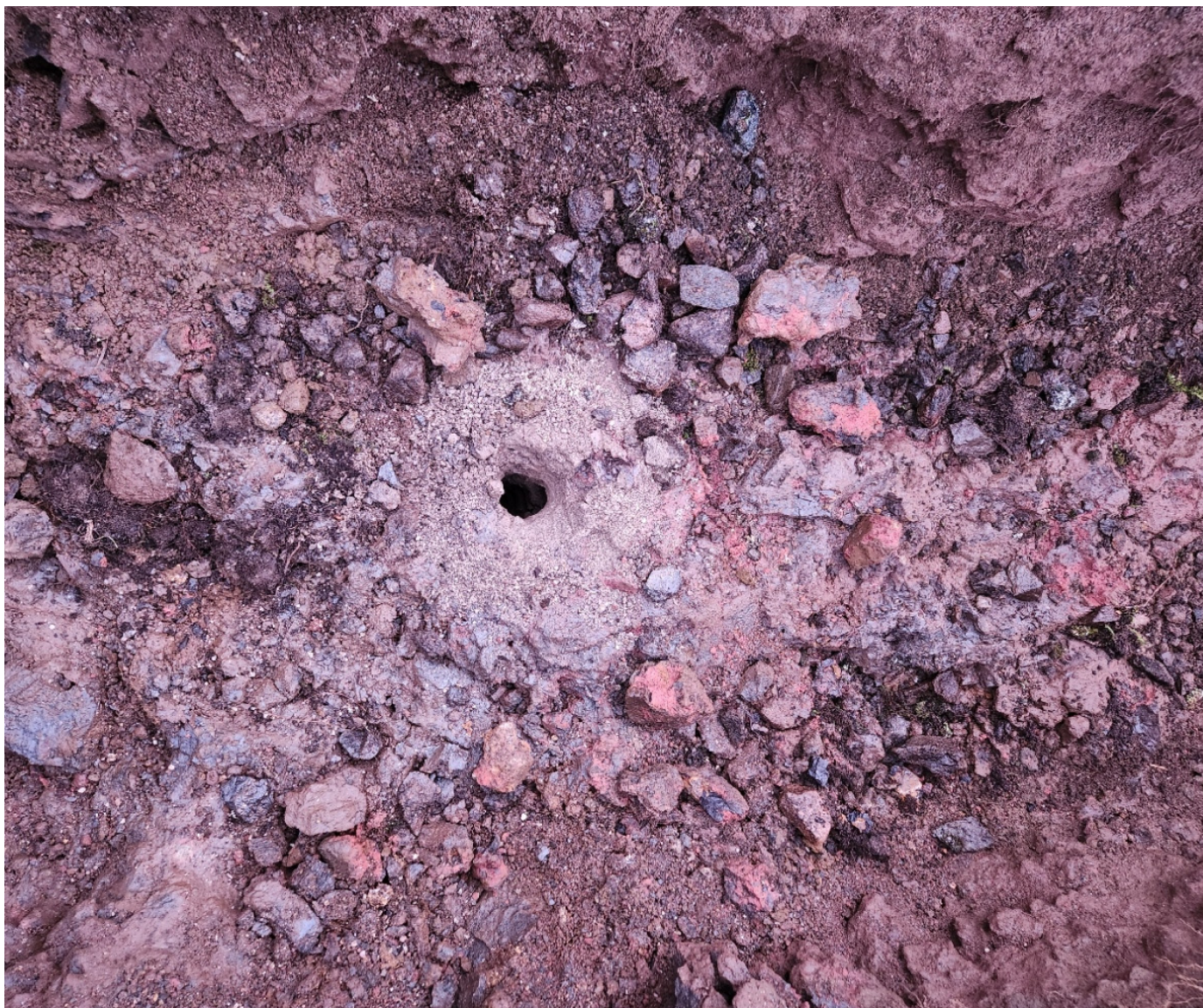
Figure 3: L5-9 Trench and drill hole image at Grønnedal showing altered magnetite with pink mineral, possible bastnasite. Similar to samples sent to St Andrews University.
